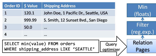
Fig. 2: A simplified example of how databases build operator trees based on user queries
